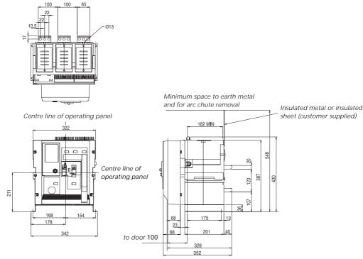
Copperwork must be supported within 200 mm of breaker connections-busbars or cables. All connections to be tightened to 50Nm. Note: Gap on both sides of the circuit breaker  $\geq$ 25mm
