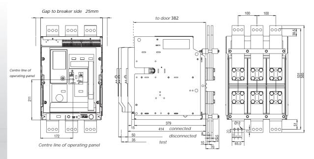
Copperwork must be supported within 200 mm of breaker connections-busbars or cables. All connections to be tightened to 50Nm.
