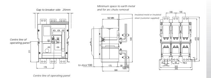
Copperwork must be supported within 200 mm of breaker connections-busbars or cables. All connections to be tightened to 50Nm.
