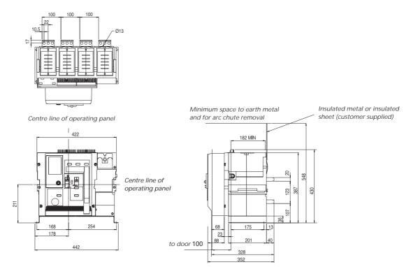
Copperwork must be supported within 200 mm of breaker connections-busbars or cables. All connections to be tightened to 50Nm. Note: Gap on both sides of the circuit breaker  $\geq$ 25mm
