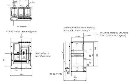
Copperwork must be supported within 200 mm of breaker connections-busbars or cables. All connections to be tightened to 50Nm.
