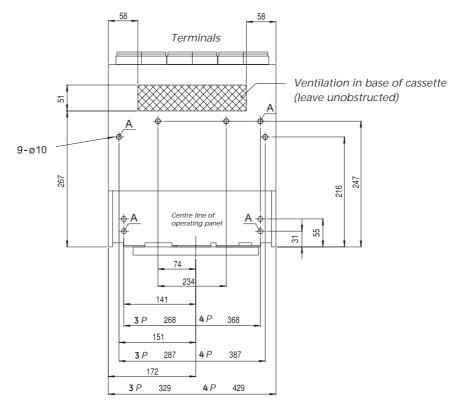
Type **A**, **D**, **In** = **3200A** to **4000A** Type **H**, **In** = **800**A to **4000A**
