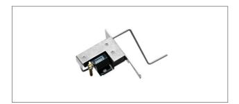
Easily fi tted, this useful accessory may be specified for use with either manual or motor charged M-PACT circuit breakers. It is clearly visible through the front panel, and the counter provides an accurate record of the cumulative number of complete breaker closing operations.
