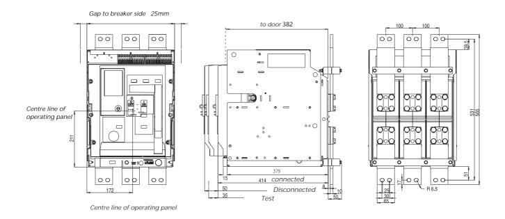
Copperwork must be supported within 200 mm of breaker connections-busbars or cables. All connections to be tightened to 50Nm.
