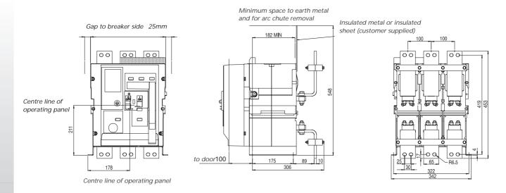
Copperwork must be supported within 200 mm of breaker connections-busbars or cables. All connections to be tightened to 50Nm.
