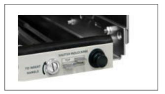
Available for withdrawable circuit breakers only, this sophisticated interlock system secures the circuit breaker in the disconnected position by means of a Ronis key. When the key is removed, the safety shutters are automatically locked in position, thus preventing access to the contacts and also ensuring that the racking mechanism is not operable. For lock and key details refer to key interlock facility section.
