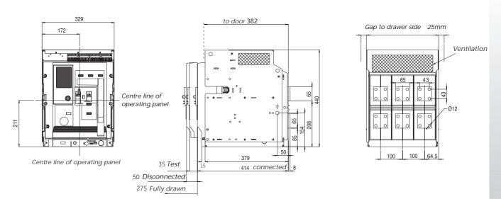
Copperwork must be supported within 200 mm of breaker connections-busbars or cables. All connections to be tightened to 50Nm.
