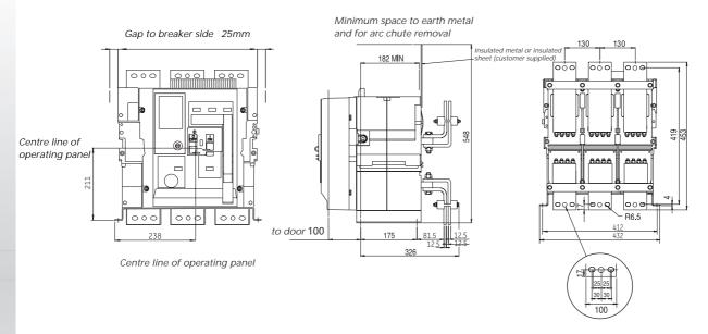
Copperwork must be supported within 200 mm of breaker connections-busbars or cables. All connections to be tightened to 50Nm.
