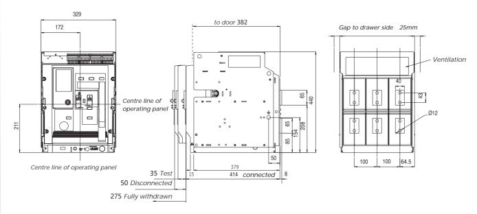
Copperwork must be supported within 200 mm of breaker connections-busbars or cables. All connections to be tightened to 50Nm.
