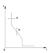
Tr Overload long-time protection time delay is applicable to cold conditions, for phase currents or neutral line currents equal to 6 Ir. When the current is greater than Isd or Ii, the tripping time takes effect according to the short delay and instantaneous protection time. Long delay minimum trip time 500ms.
