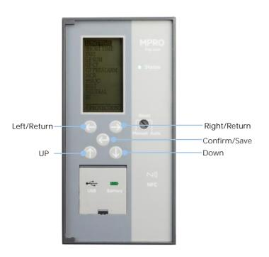
Before the device is powered on, the control unit can be activated through a power module with a standard configuration of a circuit breaker. During the normal operation of the control unit, power is supplied through the built-in induction coil of the circuit breaker or an external auxiliary power module. When there is no external power supply, the control unit is activated when the circuit breaker is loaded and the load current reaches 20% of the rated current of the circuit breaker.
