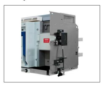
Available for fixed and withdrawable circuit breakers. These units enable the direct interlocking of M-PACT circuit breakers, either mounted side-by- side or stacked. The interlocking mechanisms are connected by a specially designed cable in '1 from 3' OR '2 from 3' configuration, and any mix of current ratings / pole confi gurations can be accommodated.
