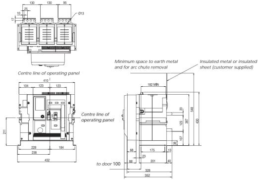
Copperwork must be supported within 200 mm of breaker connections-busbars or cables. All connections to be tightened to 50Nm.
