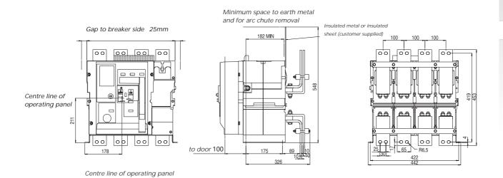
Copperwork must be supported within 200 mm of breaker connections-busbars or cables. All connections to be tightened to 50Nm.
